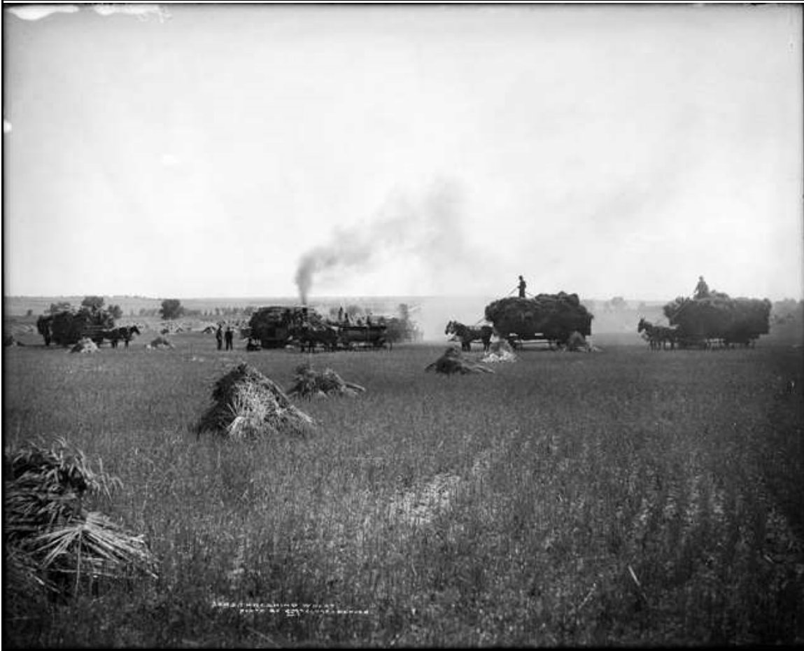
Even with increased mechanization, wheat threshing was very labor-intensive. Shown here is a steam-powered threshing machine, three horse/mule drawn wagons loaded with sheaves, and one horse-drawn water tank. Photo by L.C. McClure, ca. 1925 and 1930. Call number: MCC-3045; courtesy of Western History/Genealogy Dept., Denver Public Library.
